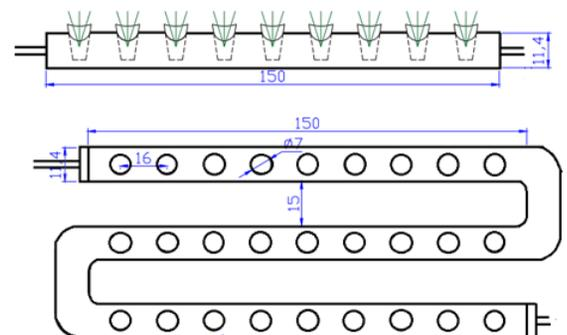
Figure 1. Hydroponic pilot (sizes in cm).
