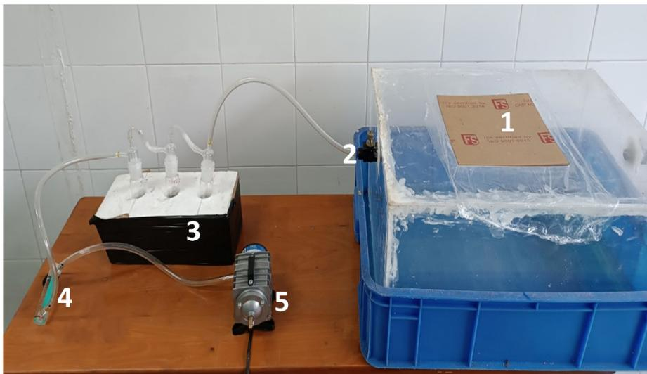
**Figure 1.** Diagram of a laboratory-scale composting system for measurement of gaseous emissions. (1) Composting tray with acrylic lid, (2) air valve, (3) three consecutive impingers, (4) rotameter, (5) air pump.
