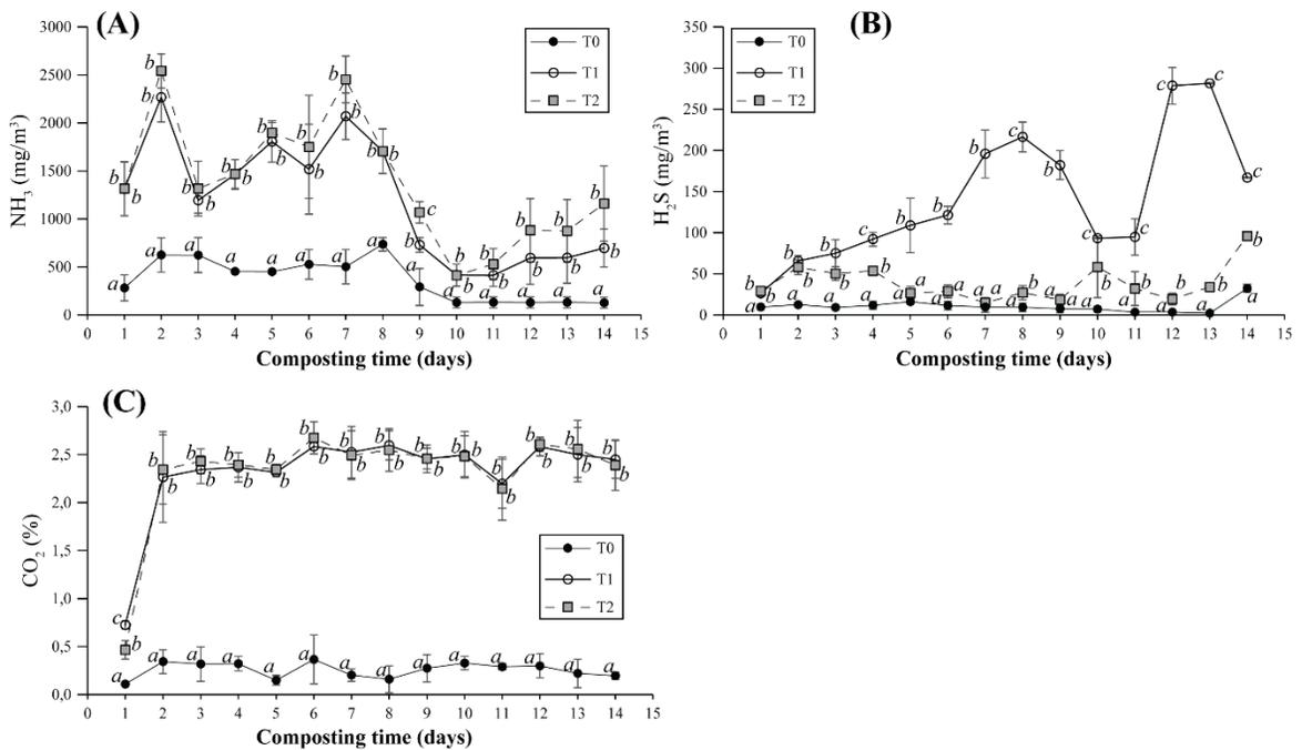
**Figure 3.** Changes of concentrations of NH<sub>3</sub> (A), H<sub>2</sub>S (B), and CO<sub>2</sub> (C) among treatments measured via the static chamber during 14-day composting of agro-waste.
