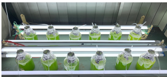
Figure 1. The photobioreactor system.
