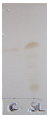
Figure 5. Chromatogram of SL analysis obtained SL; (C) standard substance (1',4"-sophorolactone 6',6"-diacetate), the Rf value is 0.55.
