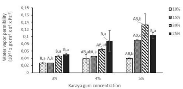
Figure 1. Effect of glycerol concentrations (10, 15, 20 and 25% w/w) on water vapor permeability of karaya films. Different letters are for significantly different groups. The capital letter (A,B) are for comparison of gum content, likewise, lower case (a,b) letters are for comparison of glycerol concentration.
