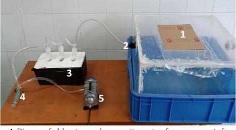
Figure 1. Diagram of a laboratory-scale composting system for measurement of gaseous emissions. (1) Composting tray with acrylic lid, (2) air valve, (3) three consecutive impingers, (4) rotameter, (5) air pump.
