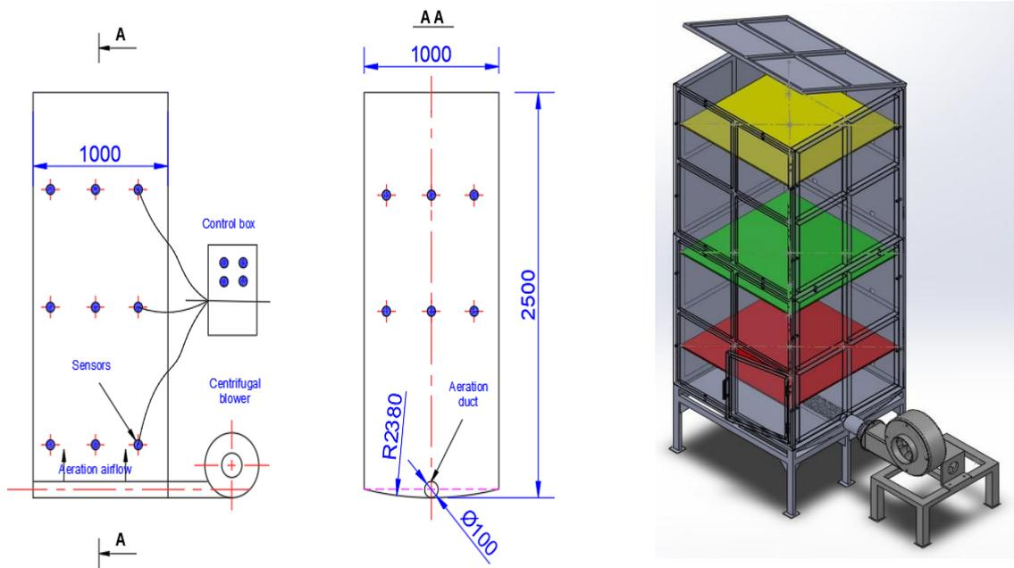
**Figure 1.** Experimental model (+ 3D) for fresh paddy aeration.
