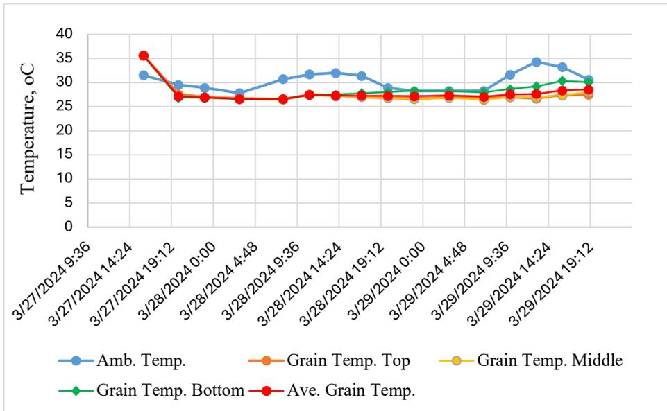
**Figure 4.** Fluctuation of aeration air and grain temperature.
